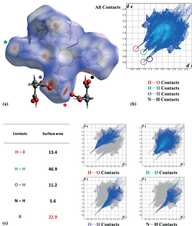
**Fig. 3** (a) Hirshfeld surface mapped on the bosentan molecule with  $d_{\text{norm}}$ . Strong contacts are pointed out and succinic acid is also represented. (b) Fingerprint plot computed from Hirshfeld surfaces. Close contacts are highlighted from inside elements: H...O (red), H...H (green), O...H (purple), and N...H (black). (c) Surface area contribution (%) of intermolecular contacts and their associated fingerprint plot regions.
