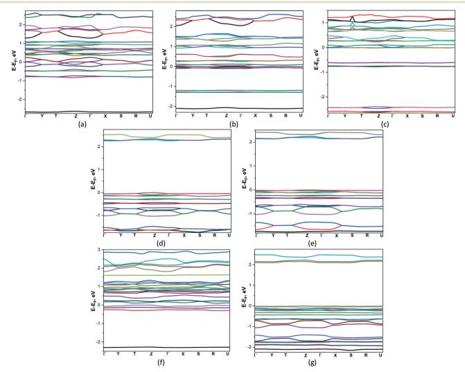
Fig. 4 Band structures compounds 1-7 (a-g). The reciprocal coordinates of high-symmetry points are  $\Gamma = (0, 0, 0), X = (0.5, 0, 0), Y = (0.5, 0, 0), Z = (0.5, 0, 0)$ = (0, 0, 0.5), S = (0.5, 0.5, 0), U = (0.5, 0, 0.5), T = (0, 0.5, 0.5), and R = (0.5, 0.5, 0.5).
