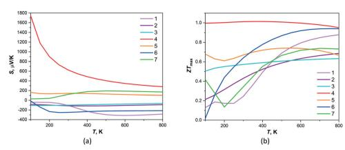
Fig. 5 Theoretical temperature dependence of (a) thermopower and (b) dimensionless figure of merit ZT calculated by BoltzTraP for compounds 1-7.
