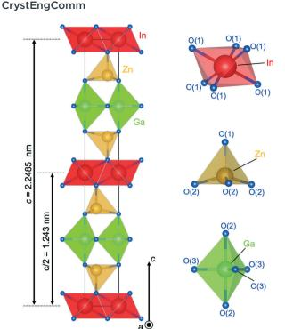
Fig. 8 Crystal structure of InGaO<sub>3</sub>(ZnO)<sub>2</sub>. Coordination of InO<sub>6</sub> octahedra, ZnO<sub>4</sub> tetrahedra, and GaO<sub>5</sub> trigonal bipyramid.
