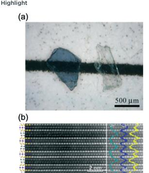
Fig. 16 (a) Single crystals of  $In_{1-x}Ga_{1+x}O_3(ZnO)_{0.5}$  before (left) and after annealing (right). (b) HAADF image with crystal structure of (InGaO<sub>3</sub>)<sub>2</sub>ZnO overlayed (left) and extracted EDX line-scan profiles for In-L (yellow), Ga-K (blue) and Zn-K (cyan) as overlay (right). Panels (a and b) are reprinted with permission from ref. 68. © 2020 Elsevier.
