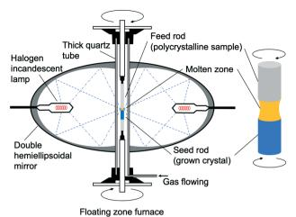
Fig. 11 Schematic image of a floating zone furnace and crystal arowth.
