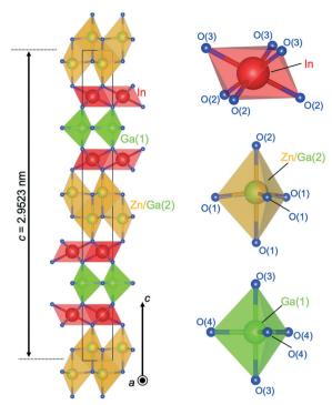
Fig. 17 Crystal structure of (InGaO<sub>3</sub>)<sub>2</sub>ZnO. Coordination of InO<sub>6</sub> is octahedra, Zn/Ga(2)O<sub>5</sub> trigonal bipyramids (two Zn/Ga(2)O<sub>4</sub> tetrahedra), and Ga(1)O<sub>5</sub> trigonal bipyramid.
