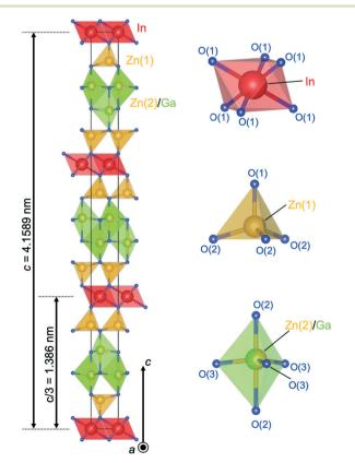
Fig. 6 Crystal structure of InGaO<sub>3</sub>(ZnO)<sub>3</sub>. Coordination of InO<sub>6</sub> is octahedra, Zn(1)O<sub>4</sub> is tetrahedra, and Zn(2)/GaO<sub>5</sub> is trigonal bipyramid.
