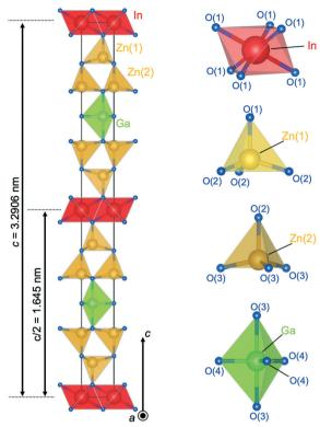
Fig. 9 Crystal structure of InGaO<sub>3</sub>(ZnO)<sub>4</sub>. Coordination of InO<sub>6</sub> octahedra, Zn(1)O<sub>4</sub> tetrahedra, Zn(2)O<sub>4</sub> tetrahedra, and GaO<sub>5</sub> trigonal bipyramid.
