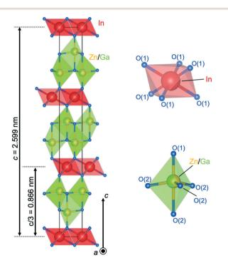
Fig. 5 Crystal structure of InGaO<sub>3</sub>(ZnO)<sub>1</sub>. Coordination of InO<sub>6</sub> is octahedra and Zn/GaO<sub>5</sub> is trigonal bipyramid. Because Zn and Ga cannot be separated, the Zn/Ga mixed site is referred to as the trigonal bipyramid in this paper.
