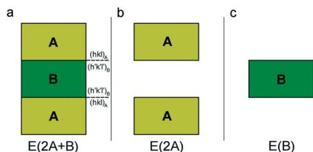
**Fig. 1** Schematic of the three systems to be optimized for calculating the adhesion energy: (a) composed slab A/B/A, (b) slab A/vacuum/A and (c) slab B. Redrawn from Bruno *et al.*<sup>1</sup>
