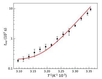
Fig. 4 Temperature dependence of the induction time for stoichiometric composition with  $[PO_4^{3-}]_0 = 0.030$  M. The solid line shows the results of modeling.
