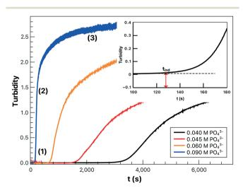
Fig. 1 Turbidity profiles for lithium phosphate at different initial reactant concentrations and (inset) the determination of induction time at 25  $^{\circ}$ C with R = 3.
