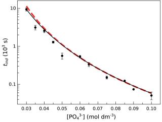
Fig. 2 Induction time as a function of initial phosphate concentration at T = 25 °C. The black solid line shows the power-law fitting according to egn (1). The red dashed line represents the calculated induction times from the kinetic model based on eqn (9)-(13).
