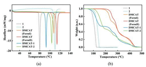
Fig. 3 (a) DSC and (b) TG patterns of the two cocrystals and their co-formers.
