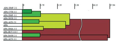
Fig. 9 Packing similarity tree diagram of APA solid forms. The horizontal axis corresponds to the PS<sub>ab</sub> value (similarity). Green indicates similar and close packing arrangements, and red indicates dissimilar packing.
