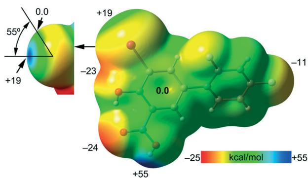
Fig. 4 MEP surface of IDIF in the *syn* conformation at the PBE0-D3/def2-TZVP level of theory. Detail of the MEP around the halogen atom is also shown (top-left) where a reduced  $\pm 19$  kcal mol $^{-1}$  energy range has been used. The energies at selected points of the surface are given in kcal mol $^{-1}$ .
