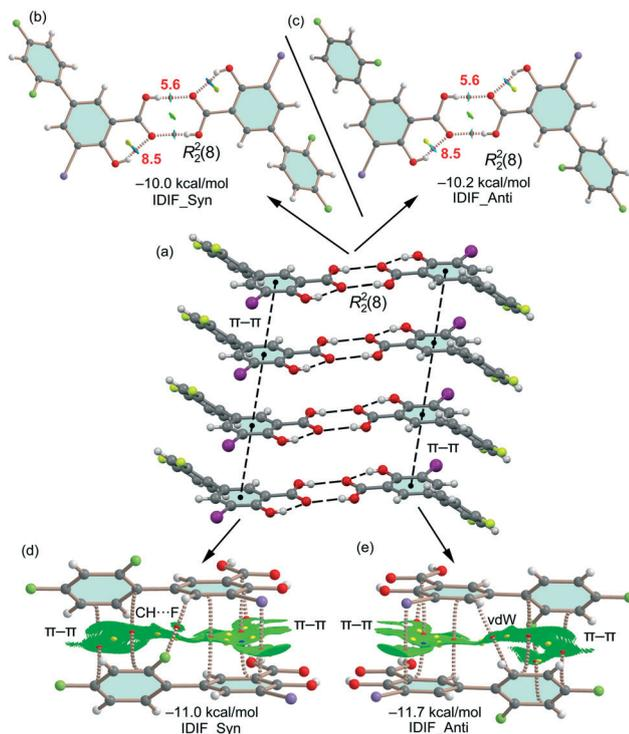
**Fig. 5** (a) Partial view of the crystal structure of IDIF. Distances in Å. (b–e) QTAIM analysis of intermolecular bond, ring and cage CPs (red, yellow and blue spheres, respectively) and bond paths of the two dimers of IDIF. For the  $R_2^2(8)$  dimer, the CP characterizing the intramolecular OH...O H-bonds are also shown. The dissociation energies are indicated in red next to the bond CPs.
