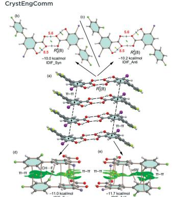
Fig. 5 (a) Partial view of the crystal structure of IDIF. Distances in Å. (b-e) QTAIM analysis of intermolecular bond, ring and cage CPs (red, vellow and blue spheres, respectively) and bond paths of the two dimers of IDIF. For the R<sub>2</sub>(8) dimer, the CP characterizing the intramolecular OH···O H-bonds are also shown. The dissociation energies are indicated in red next to the bond CPs.
