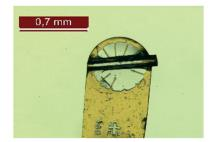
Fig. 7 Crystal of compound 3 analysed by single crystal diffraction.
