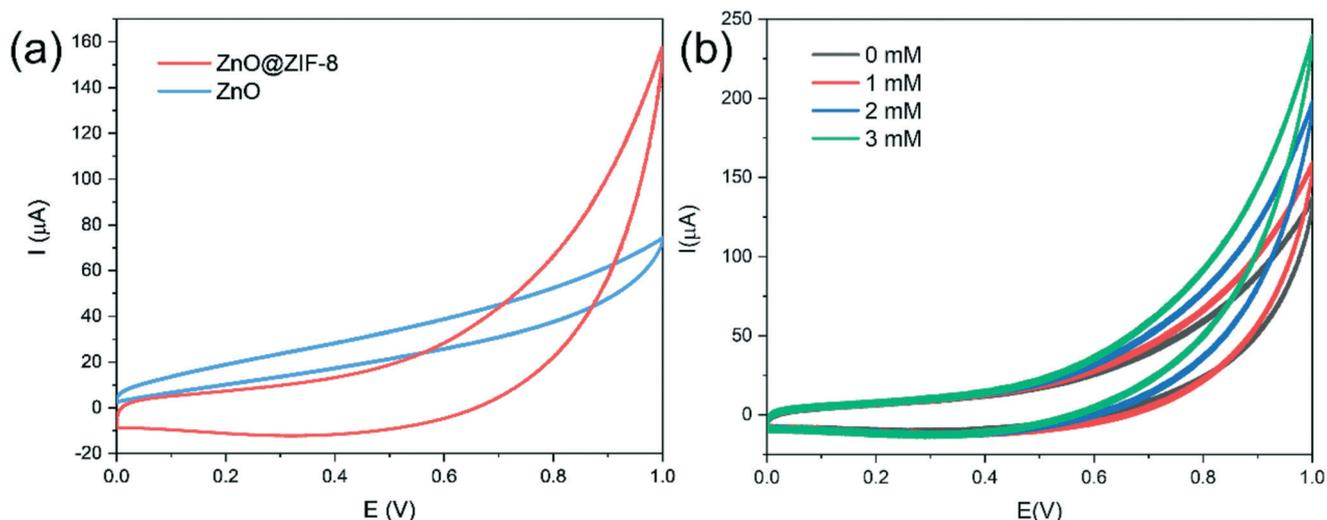
Fig. 5 (a) Cyclic voltammograms of the ZnO nanorod arrays and the ZnO@ZIF-8 nanorod arrays in the presence of 1 mM H<sub>2</sub>O<sub>2</sub> in PBS (0.1 M, pH 7.0) at a scan rate of 50 mV s<sup>-1</sup>; (b) cyclic voltammograms of ZnO@ZIF-8 nanorod arrays in PBS including various concentrations of H<sub>2</sub>O<sub>2</sub> at 50 mV s<sup>-1</sup>.
