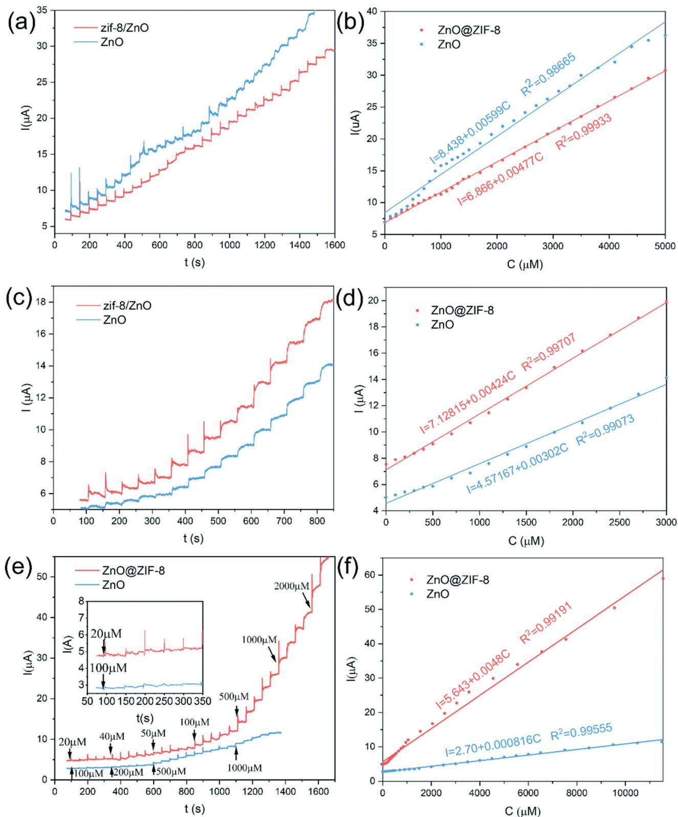
Fig. 6 The current response of ZnO and ZnO@ZIF-8 nanorod arrays to successive addition of H<sub>2</sub>O<sub>2</sub> in PBS (0.1 M, pH 7.0) at an applied potential of 0.6 V on the first day (a and b), the seventh day (c and d) and the twenty-first day (e and f).
