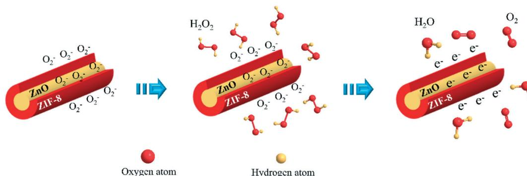
**Fig. 7** Sensing mechanism of ZnO@ZIF-8 nanorod arrays.
