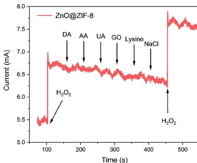
**Fig. 8** Amperometric response of ZnO@ZIF-8 nanorod arrays to the addition of 0.3 mM H<sub>2</sub>O<sub>2</sub> or 0.1 mM other interferents in PBS (0.1 M, pH = 7.0) at an applied potential of 0.6 V.
