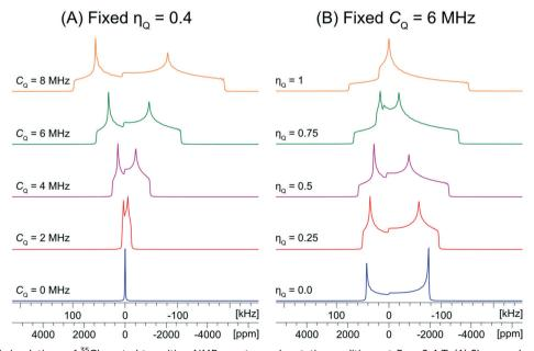
Scheme 1 Analytical simulations of  $^{35}$ Cl central transition NMR spectra under static conditions at  $B_0 = 9.4$  T. (A) Shows values of  $C_Q$  ranging from 0 to 8 MHz with a fixed  $\eta_Q$  = 0.4 and (B) shows values of  $\eta_Q$  ranging from 0 to 1 with a fixed  $C_Q$  = 6 MHz. The range of  $C_Q$  values is selected to be representative of those typically observed for chloride ions.
