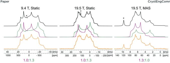
Fig. 5 Experimental <sup>35</sup>Cl(<sup>1</sup>H) SSNMR spectra of NH<sub>4</sub>Cl:Urea (lower traces), corresponding analytical simulations (upper traces), and deconvolutions of the simulations (middle traces). Spectra were acquired at two fields ( $B_0 = 9.4$  T and 19.5 T) under static and MAS conditions ( $v_{rot} = 16$  kHz). Peaks corresponding to NH<sub>4</sub>Cl educt are indicated with asterisks (\*).
