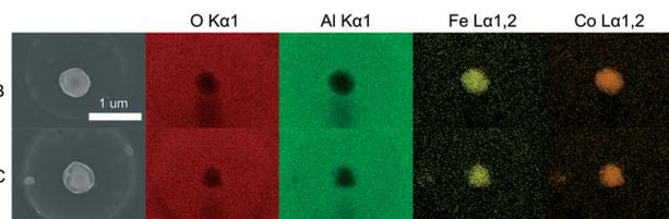
Fig. 11 EDX elemental analysis maps of the two crystals (B and C) shown in Fig. 10. Shown are 2D signals for the substrate,  $\text{Al}_2\text{O}_3$ , and primary Co-Fe emission lines. The maps were collected using a ZEISS Merlin analytical SEM equipped with an in-lens detector with an acceleration voltage of 10 kV.
