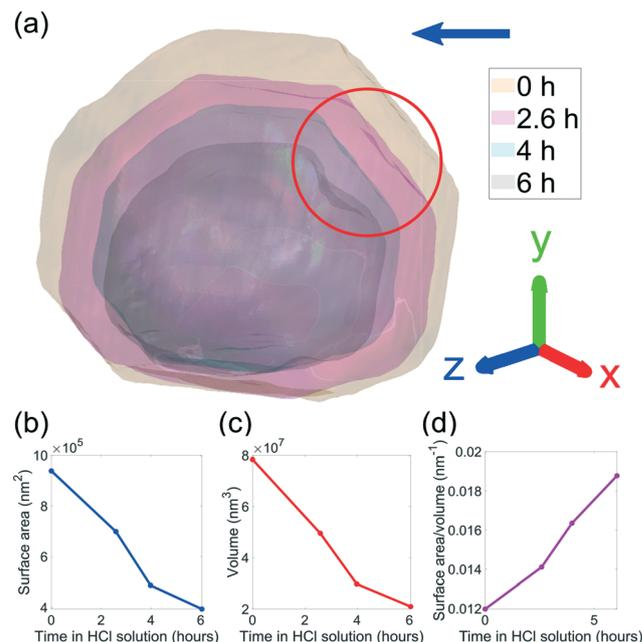
**Fig. 4** (a) Translucent morphologies of the (111) reconstructions as a function of corrosion time. The red circle highlights the formation of a pit on the (100) facet. The blue arrow shows the direction of fluid flow. The amplitude threshold is 0.25 and the magnitude of the coordinate axes corresponds to 100 nm. (b–d) The evolution of volume, surface area, and surface area to volume ratio of the crystal as a function of corrosion time, respectively.
