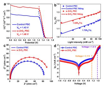
Fig. 3 (a) C-V curves, (b) dependence of  $V_{\rm oc}$  on light intensity, (c) EIS spectra, and (d) dark J-V curves of control and  $ZrO_2$ -capped CsPbIBr<sub>2</sub> PSCs.
