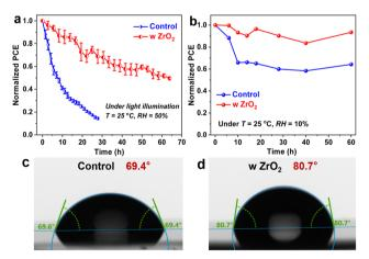
Fig. 4 (a and b) Stability levels of unencapsulated control and ZrO2capped PSCs under (a) persistent light irradiation and (b) dry air conditions. The errors in the data (indicated by error bars) originate from the fluctuation of the light intensity of the xenon lamp. (c and d) Contact angles of water on perovskite films before and after they were capped with a ZrO<sub>2</sub> laver at T = 25 °C and RH = 50%.
