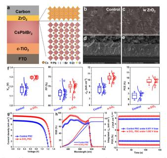
Fig. 1 (a) Illustration of the structure of the ZrO<sub>2</sub>-capped device. (b and c) Top-view SEM images of perovskite films with and without the ZrO2 capping layer. (d and e) Cross-sectional SEM images of the PSCs. (f) Statistical photovoltaic parameters of control and optimal PSCs. (g) J-V curves, (h) EQE spectra and (i) steady power output curves of control and optimal PSCs.
