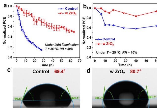
Fig. 4 (a and b) Stability levels of unencapsulated control and  $ZrO_2$ -capped PSCs under (a) persistent light irradiation and (b) dry air conditions. The errors in the data (indicated by error bars) originate from the fluctuation of the light intensity of the xenon lamp. (c and d) Contact angles of water on perovskite films before and after they were capped with a  $ZrO_2$  layer at  $T = 25$  °C and  $RH = 50\%$ .
