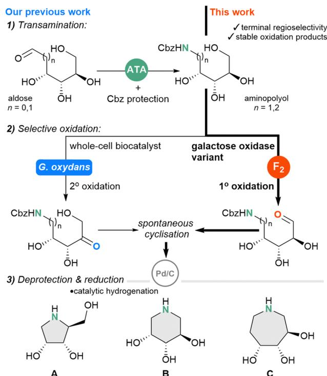
**Scheme 1** Biocatalytic routes to pyrrolidine-(A), piperidine-(B) and azepane-(C) type iminosugars from monosaccharides. Previous work includes transamination<sup>12</sup> and *G. oxydans* mediated secondary oxidation<sup>20</sup> ATA = amine transaminase, F<sub>2</sub> = galactose oxidase variant F<sub>2</sub>.
