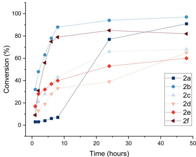
Fig. 1 Time course analysis of the GOase F<sub>2</sub>-catalysed oxidation of N-Cbz-protected aminopolyols. Conversion to products **2a–f** was determined by LC/MS analysis, monitoring product formation at timepoints up to 48 hours, and plotted as the average of triplicate reactions (1 mL) (for individual plots with error bars, see ESI,† Section 4).
