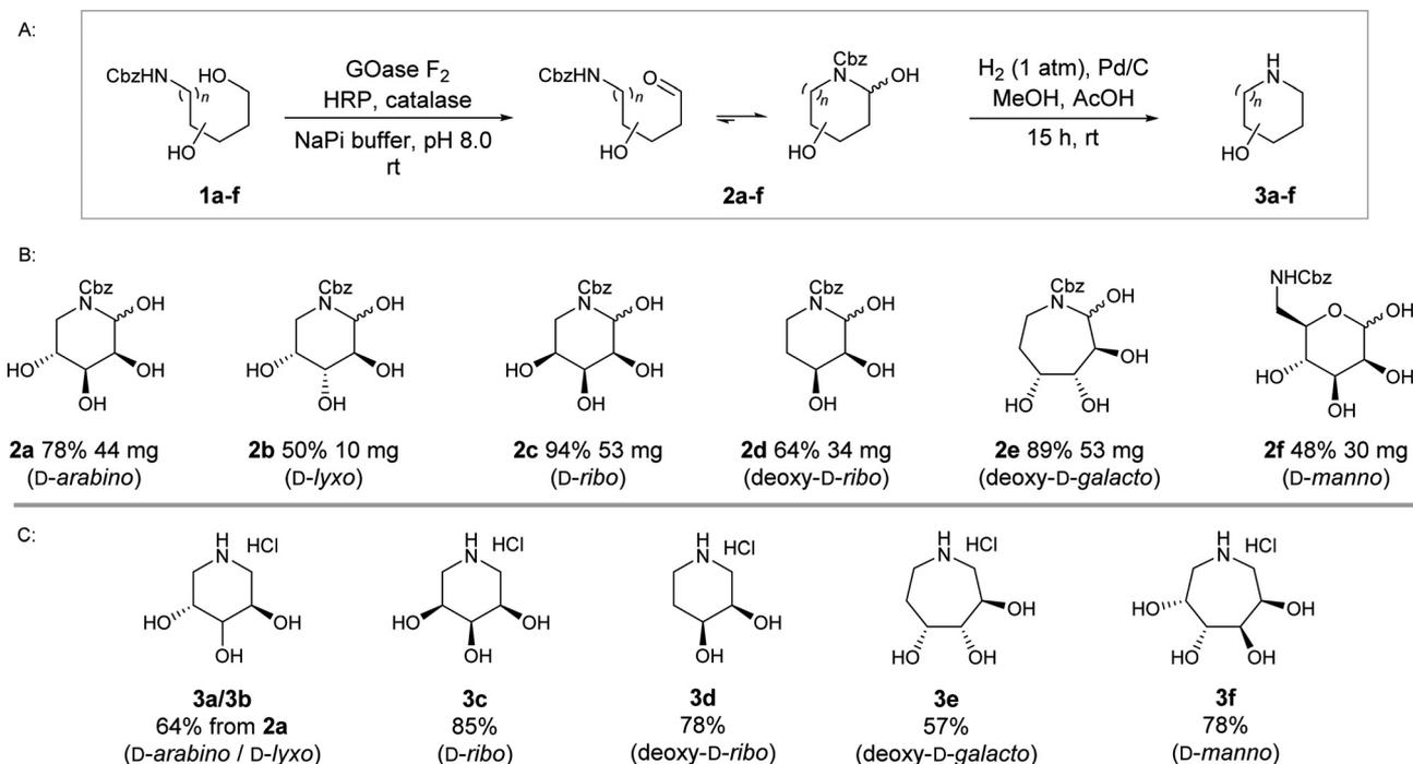
**Scheme 2** (A) Chemoenzymatic synthesis of piperidine- and azepane-type iminosugars. (B) Substrate scope of the oxidation products and isolated yields, products **2a–e** exist predominantly in hemiaminal form, whereas **2f** is in hemiacetal form. (C) Iminosugars **3a–f** are isolated as the HCl salt.
