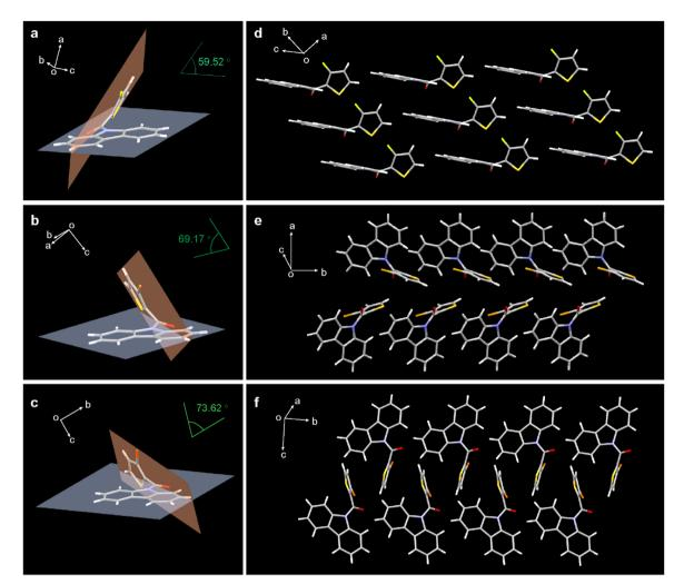
Fig. 3 Probable explanation of different photo-acid quantum yeilds and melting points. Dihedral Angle between carbazole plane and thiophene plane of (a) CzF, (b) CzCl, and (c) CzBr. The packing modes of crystals of (d) CzF, (e) CzCl. and (f) CzBr.
