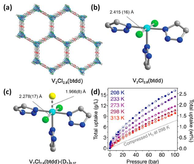
**Fig. 6** (a) The 3D structure of V<sub>2</sub>Cl<sub>2.8</sub>(btdd) and the coordination environment of the V(II) centre in (b) the activated framework and (c) in the framework dosed with 0.75 equiv. of D<sub>2</sub> molecules. (d) The high-pressure H<sub>2</sub> isotherm in the temperature range of 208–313 K. Reprinted with permission from ref. 56. Copyright 2021, American Chemical Society.
