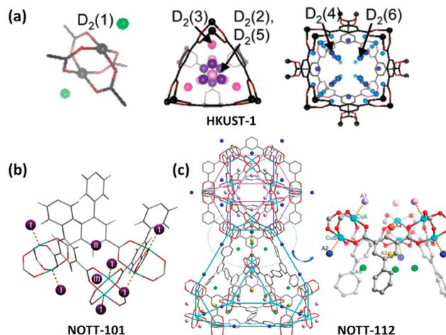
Fig. 5 D<sub>2</sub> binding sites in copper-multicarboxylate frameworks of (a) HKUST-1, (b) NOTT-101 and (c) NOTT-112 compounds as determined by the NPD experiment with D<sub>2</sub> loadings of 4, 1.82 and 2.0 per copper ion, respectively. Reprinted with permission from ref. 42 and 43. Copyright 2006, and 2009–2010, American Chemical Society.
