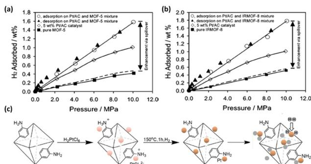
Fig. 10 Comparison of H<sub>2</sub> isotherms of (a) MOF-5 and (b) IRMOF-8 before and after Pt doping exhibiting significantly enhanced H<sub>2</sub> storage capacities via the spillover effect. (c) Schematic representation of the synthetic route of Pt/aUiO that can dissociate dihydrogen to hydrogenate the organic linker. Reprinted with permission from ref. 80 and 81. Copyright 2006 and 2021, American Chemical Society.
