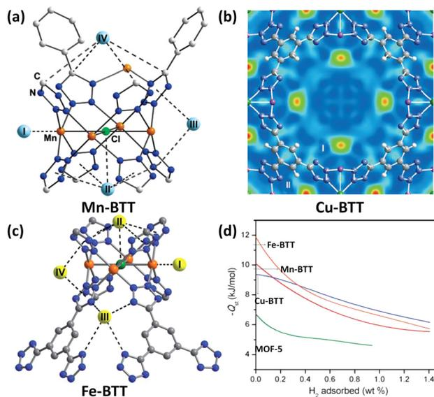
Fig. 4  $D_2$  binding sites in (a) Mn-BTT, (b) Cu-BTT and (c) Fe-BTT compounds as determined by the NPD experiment with the  $D_2$  loadings of 12, 30 and 20 per formula unit, respectively, and (d) comparison of their  $H_2$  adsorption heats. Reprinted with permission from ref. 36, 38 and 39. Copyright 2006, American Chemical Society; Copyright 2007, Wiley; Copyright 2010, Royal Society of Chemistry.
