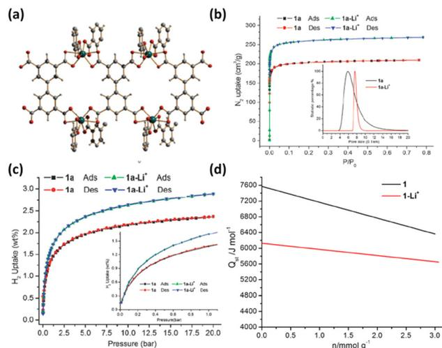
Fig. 9 (a) The partial structure of  $(\text{Me}_2\text{NH}_2)[\text{In}(\text{L})]$  and comparison of (b)  $\text{N}_2$  and (c)  $\text{H}_2$  isotherms at 77 K and (d)  $\text{H}_2$  adsorption heat for  $(\text{Me}_2\text{NH}_2)[\text{In}(\text{L})]$  before and after  $\text{Li}^+$  exchange. Reprinted with permission from ref. 70. Copyright 2008, Royal Society of Chemistry.
