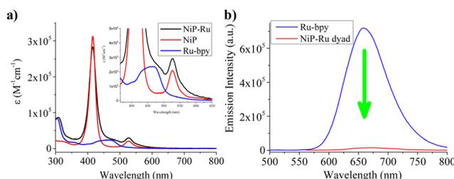
**Fig. 1** (a) Absorption spectrum of **NiP-Ru** dyad, **NiP** and **Ru-bpy** in DMF, (b) Emission intensity of **Ru-bpy** (blue line) and **NiP-Ru** dyad (red line) after excitation at 480 nm, recorded in DMF solutions with a concentration of 0.01 mM of individual compounds.
