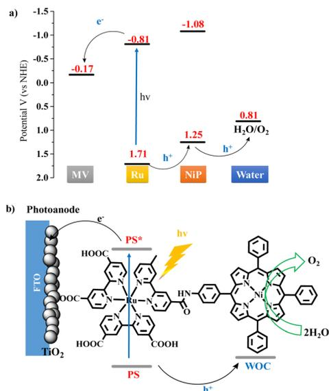
**Scheme 1** (a) Energy diagram of the **NiP-Ru-bpy** dyad derived photo-induced electron transfer process resulting in water oxidation. (b) Schematic diagram of the visible light-driven water oxidation by the **NiP-Ru** dyad modified  $\text{TiO}_2/\text{FTO}$  photoanode.
