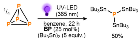
Scheme 3 Initial conditions for the direct, photocatalytic stannylation of P_4 into (Bu_3Sn)_3P optimized using benzophenone ( BP ) as photocatalyst. Stoichiometries in equiv. and mol% are defined per P atom.
