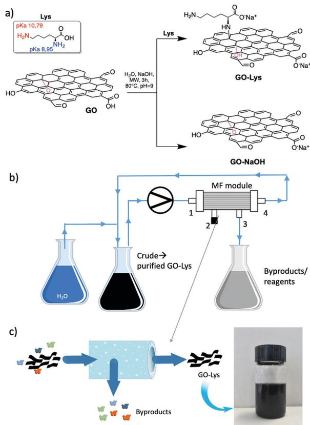
**Scheme 1** (a) Synthetic route to GO-Lys and GO-NaOH, (b) sketch of the purification of GO-Lys by microfiltration, and (c) zoomed-in view of the microfiltration procedure and image of the GO-Lys suspension ( $2 \text{ mg mL}^{-1}$  after 30 h from sonication).
