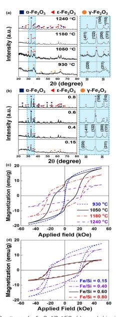
Fig. 2 XRD patterns of  $\epsilon$ -Fe<sub>2</sub>O<sub>3</sub> NPs@SiO<sub>2</sub> (a) annealed in air at various temperatures for 4 h using precursor particles with a precursor molar ratio (Fe/Si) of 0.4:1 and (b) prepared using various precursor molar ratios (Fe/ Si) under the optimized annealing conditions (1180  $^{\circ}$ C, 4 h) and (c) and (d) magnetic hysteresis loops of  $\varepsilon$ -Fe<sub>2</sub>O<sub>3</sub> NPs in (a) and (b) after SiO<sub>2</sub> removal.
