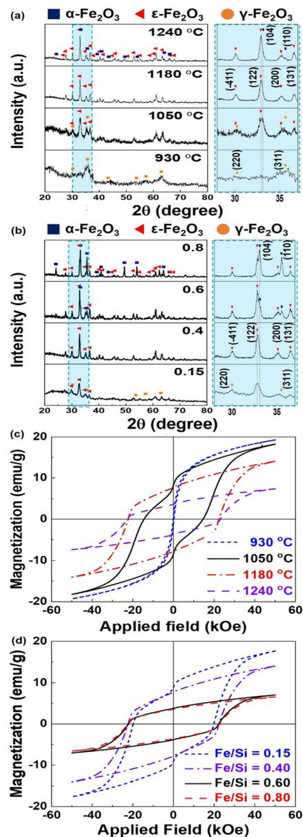
Fig. 2 XRD patterns of  $\epsilon$ - $\text{Fe}_2\text{O}_3$  NPs@ $\text{SiO}_2$  (a) annealed in air at various temperatures for 4 h using precursor particles with a precursor molar ratio (Fe/Si) of 0.4 : 1 and (b) prepared using various precursor molar ratios (Fe/Si) under the optimized annealing conditions (1180 °C, 4 h) and (c) and (d) magnetic hysteresis loops of  $\epsilon$ - $\text{Fe}_2\text{O}_3$  NPs in (a) and (b) after  $\text{SiO}_2$  removal.
