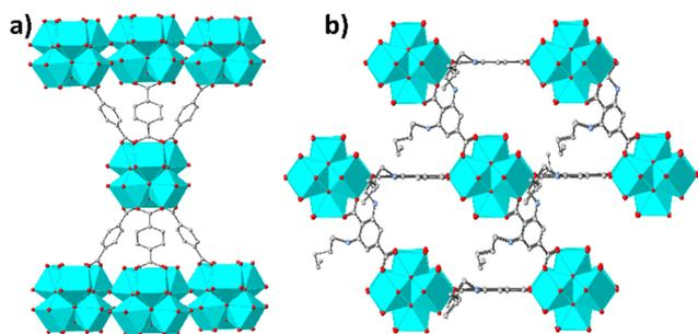
Fig. 2 Representation of (a) the cluster connectivity and (b) framework structure of **HEX-MOF** (C, gray; O, red; N, blue; and Zr turquoise), as obtained *via* the Rietveld refinement. The H atoms and the solvent molecules in the structural representation of **HEX-MOF** were omitted for clarity.
