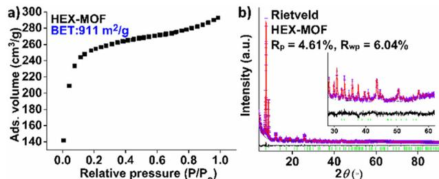
Fig. 1 (a)  $N_2$  sorption isotherm (77 K) for **HEX-MOF**. (b) Rietveld plot of **HEX-MOF**. Violet crosses: experimental points; red line: calculated pattern; black line: difference pattern (exp-calc); and green bars: Bragg positions. Inset: Magnification of the  $2\theta$  region  $30\text{--}60^\circ$ .
