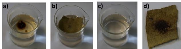
Fig. 5 (a) Crude oil in water sample, (b) sorption of crude oil on **HEX-MOF@cotton fabric**, (c) oil-free water (obtained after the treatment with the fabric sorbent), (d) **HEX-MOF@cotton fabric** after crude oil sorption.
