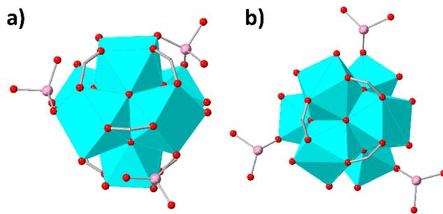
Fig. 4 The coordination mode of (a) As(V) and (b) As(III) species (Arsenic atoms shown as pink balls) in the structures of **HEX-MOF/As(V)** and **HEX-MOF/As(III)** respectively, as determined *via* Rietveld refinement.
