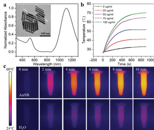
**Fig. 1** (a) UV-Vis absorption spectra and TEM of AuNRs. (b) Photothermal activity of AuNRs with different concentrations under 1064 nm laser irradiation ( $1 \text{ W cm}^{-2}$ ). (c) Thermal images of AuNR solutions and pure H<sub>2</sub>O after irradiating for 0, 2, 4, 6, 8 and 10 min.
