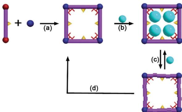
**Fig. 3** A regenerative MOF for reversible uptake of  $\text{Cd}(\text{II})$ : (a) self assembly 3D framework from organic ligand and hard metal ion; (b) effective absorption with high capacity; (c) absorption and desorption; (d) reconstruction of the used sample into a fresh sample. Reproduced from ref. 96 with permission from Royal Society of Chemistry, copyright 2016.
