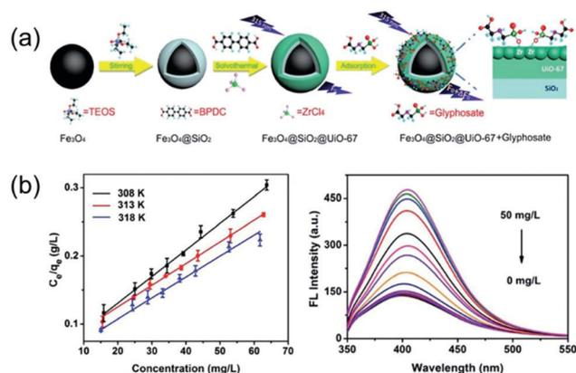
Fig. 11 (a) A schematic illustration of the fabrication of the Fe<sub>3</sub>O<sub>4</sub>@SiO<sub>2</sub>@UiO-67 MOF-based adsorbent. (b) The adsorption and the detection performance for glyphosate treatment. Reproduced from ref. 147 with permission from Royal Society of Chemistry, copyright 2018.
