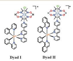
Scheme 1 Structure of the Ir-Co based dyads I and II obtained respectively through chelation of the Ir-based photosensitizers [Ir(ppy)2-L] and [Ir(piq)2-L] with the Co-based catalyst.
