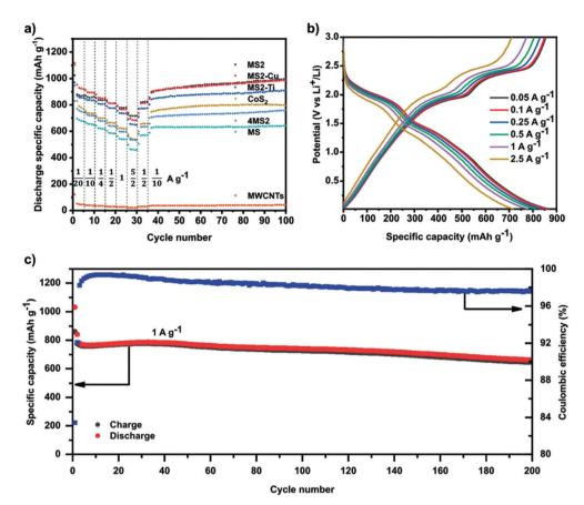
Fig. 6 (a) Galvanostatic rate performance test of all HESs,  $CoS_2$ , 4MS2, and MWCNTs half-cell at different current densities and 25 °C in the voltage range between 0.01 and 3 V versus Li<sup>+</sup>/Li. (b) Voltage profiles of MS2 half-cell at different currents. (c) Specific charge/discharge capacity of  $MS_2$  half-cell and Coulombic efficiency as a function of cycle number at 1 C and 25 °C in the range between 0.01 and 3 V. Copyright permission from Wiley, used from ref. 52.
