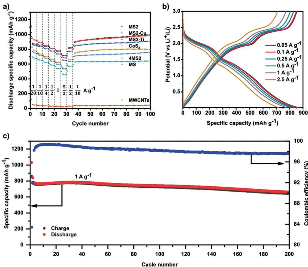
Fig. 6 (a) Galvanostatic rate performance test of all HESSs,  $\text{CoS}_2$ , 4MS2, and MWCNTs half-cell at different current densities and 25 °C in the voltage range between 0.01 and 3 V versus  $\text{Li}^+/\text{Li}$ . (b) Voltage profiles of MS2 half-cell at different currents. (c) Specific charge/discharge capacity of MS2 half-cell and Coulombic efficiency as a function of cycle number at 1 C and 25 °C in the range between 0.01 and 3 V. Copyright permission from Wiley, used from ref. 52.
