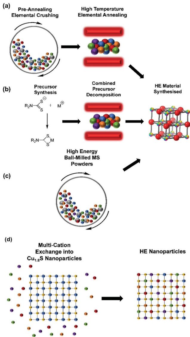
Fig. 3 Figure showing a schematic representation of extant synthetic procedures toward high entropy metal chalcogenides. (a) elemental annealing (b) thermolysis of single source precursor cocktails (c) high energy ball-milling of individual metal sulphides (d) nanoparticle cation exchange.
