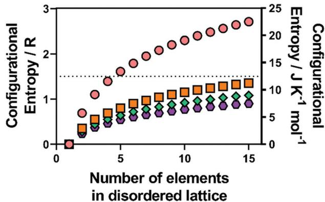
Fig. 1 Calculated configurational entropy (in both R and  $\text{J K}^{-1} \text{mol}^{-1}$ ) for species with a single disordered sub-lattice (M) for (pink circles) alloys with a single lattice, and a range of common metal chalcogenide materials with a single chalcogenide sub-lattice (*i.e.* X is all O, S, Se or Te) for (orange squares) MX, (blue diamonds)  $\text{M}_2\text{X}_3$  and (purple hexagons)  $\text{MX}_2$ .
