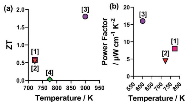
Fig. 7 Figure showing the reported *zT* and power factor (PF) values for non-oxide HE metal chalcogenides. Where [1] Cu<sub>5</sub>Sn<sub>1.2</sub>MgGeZnS<sub>9</sub>, [2], (CoFeNi)(SSe), [3] (PbSbSn)(SSeTe), [4] (AgPbBi)(SSeTe) correspond to ref. 37, 47, 54 and 66.
