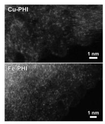
Fig. 2 Annular dark-field scanning transmission electron microscopy images of Cu-PHI and Fe-PHI, where bright dots correspond to highly dispersed metal atoms
