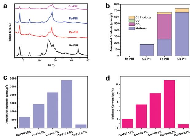
**Fig. 1** (a) Powder XRD patterns of M-PHI; (b) distribution of products of methane photooxidation with Na, Co, Fe and Cu-PHI (10% of metal loading); (c) influence of metal loading in Cu-PHI samples for methanol production; (d) methane conversion in different Cu loadings in PHI.
