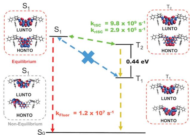
Fig. 5 NTOs for the  $S_1$ ,  $T_1$  and  $T_2$  states and schematics of the TADF mechanism in compound **1** with DFT estimated rates in toluene. A CT  $S_1$  state calculated at a non-equilibrium geometry is also shown.
