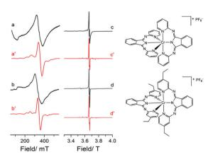
Fig. 2 Experimental and simulated EPR spectra of (a and c)  $[Cr(\mathbf{bpi-1})_2]PF_6$  and (b and d)  $[Cr(\mathbf{bpi-2})_2]PF_6$  recorded as 1% doped solids in their corresponding diamagnetic cobalt matrix. Experimental data were recorded at (a and b) X-band frequency, 140 K, and (c and d) W-band frequency, 20 K.
