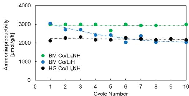
Fig. 5 Cyclability tests of Co/LiH and Co/Li<sub>4</sub>NH samples. Reaction conditions for one cycle: 60 sccm N<sub>2</sub> followed by 75 sccm H<sub>2</sub>, 1 barg, 450 °C, 15 mg material. HG = hand-ground, BM = ball-milled.
