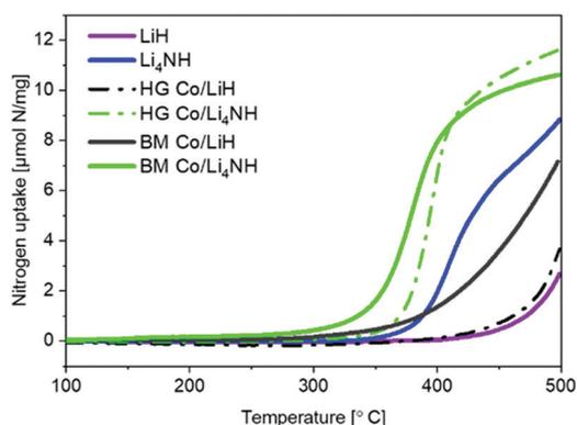
**Fig. 2** N<sub>2</sub>-TPR profiles of plain and cobalt-composited LiH and Li<sub>4</sub>NH. HG = hand-ground, BM = ball-milled.
