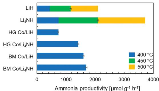
**Fig. 1** Ammonia synthesis rate with plain LiH, Li<sub>4</sub>NH and cobalt-containing samples in a chemical looping process. Reaction conditions: 60 sccm N<sub>2</sub> followed by 75 sccm H<sub>2</sub>, 1 barg, 20 mg material. The stacked bars at 450 and 500 °C for LiH and Li<sub>4</sub>NH show the absolute rate and not the increase in rate from that observed at the lower temperature. HG = hand-ground, BM = ball-milled.
