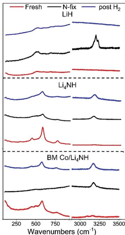
Fig. 4 The low-energy phonon vibration region and the N–H stretching region of the Raman spectra of LiH, Li<sub>4</sub>NH and BM Co/Li<sub>4</sub>NH samples.
