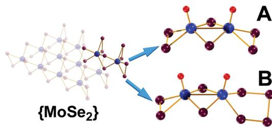
Fig. 1 Ball-and-stick representation of: (A)  $[\text{Mo}_2\text{O}_2(\mu\text{-Se})_2(\text{Se}_2)_2]^{2-}$  and (B)  $[\text{Mo}_2\text{O}_2(\mu\text{-Se})_2(\text{Se}_2)(\text{Se}_4)]^{2-}$ . Colour code: Mo, Blue; Se, plum; O, red; Counterions are omitted for clarity.
