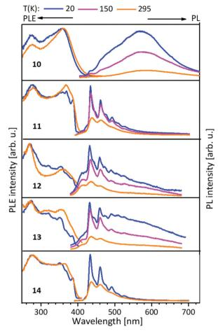
Fig. 7 Solid state excitation and emission spectra of NHC $^{impy}$  ( $L^3$ ) metal complexes 10–14. PL was excited at  $\lambda_{\rm exc}$  = 350 nm and PLE spectra recorded at  $\lambda_{em}$  = 580 nm for **10** and  $\lambda_{em}$  = 430 nm for **11–14**,  $\lambda_{em}$  = 430/ 460 nm (13).43
