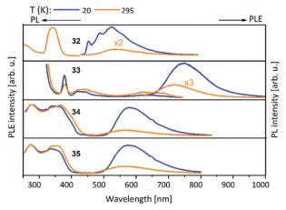
Fig. 10 Solid state excitation and emission spectra of PN<sub>4</sub> (L<sup>12</sup>) metal complexes **32–35**. PL was excited at  $\lambda_{\rm exc}$  = 350 nm and PLE spectra recorded at  $\lambda_{em}$  = 560 nm for **32**, **33**, **35** and  $\lambda_{em}$  = 580 nm for **34**. <sup>48</sup>
