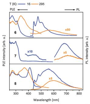
Fig. 6 Solid state excitation and emission spectra of bis-NHCbipy (L2) metal complexes 6-8. PL was excited at  $\lambda_{exc}$  = 300 nm for 6, 8 and  $\lambda_{\rm exc}$  = 320 nm for **7**. PLE spectra were recorded at  $\lambda_{\rm em}$  = 500/560 nm (**6**),  $\lambda_{em}$  = 700/750 nm (7) and  $\lambda_{em}$  = 550/600 nm (8) at low/elevated temperatures respectively.42
