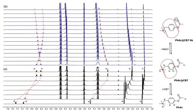
Fig. 3 (a) NMR titration experiments of free **PhAc** (1.5 mM) with **CB7** (0–1.65 mM) and (b) the **PhAc@CB7** complex (2.0–1.4 mM) with NaCl (0–460 mM). The concentration of **CB7** and NaCl increases from the bottom up. The signals of two aromatic hydrogen atoms 2c and 3c coalesce at the concentration of NaCl equal to 10 mM.
