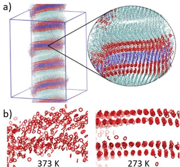
Fig. 5 (a) MD snapshot of the lamellar structure formed by the HOB-10-HOB compound. Cyan, red and blue sticks represent oleyl chains, aromatic rings, and linkers. (b) Snapshots of the MD showing the configuration adopted by the aromatic moieties in the assembled structure formed by the HOB-10-HOB at different temperatures.
