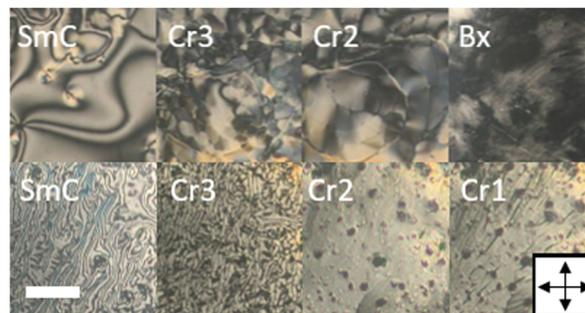
**Fig. 2** POM images at temperatures corresponding to different phases of representatives of even (upper) and odd (lower) HOB-*n*-HOB. Scale bar represents 60 μm. Other XRD and POM results are shown in Fig. S2 and S3 (ESI†).
