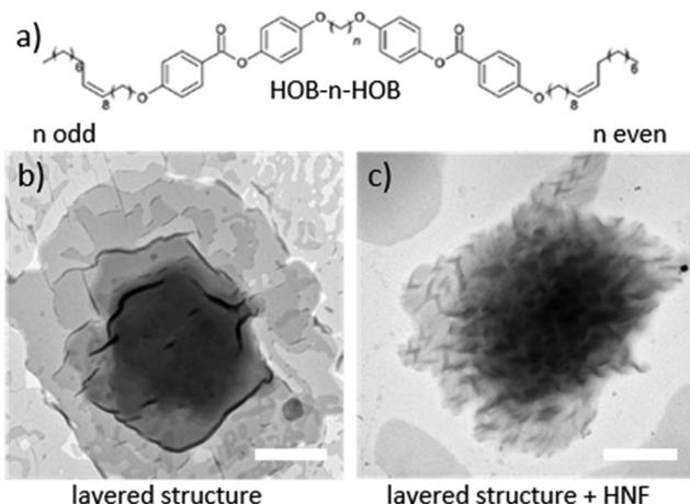
**Fig. 1** Odd–even effect in HOB-*n*-HOB series. (a) Structure of HOB-*n*-HOB and shape of its most stable conformers for odd and even values of *n*, TEM images of (b) layered structures formed by HOB-11-HOB and (c) helical (twisted layered) structures formed by HOB-12-HOB. Scale bars represent 500 nm.
