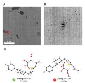
Fig. 2 (A) TEM image of microcrystals of API 1-D-malate. The target used for diffraction is shown in red. (B) The corresponding MicroED diffraction pattern. (C) The two potential configurations of the structure with the correct configuration indicated
