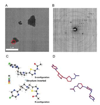
Fig. 1 (A) TEM image of a microcrystal of API 1. The target used for diffraction is shown in red. (B) The corresponding MicroED diffraction pattern. (C) One molecule of API 1 from the MicroED structure is shown in the two possible absolute configurations. Either configuration fits the experimental data equally well. (D) An overlay of the MicroED (blue) and scXRD (red) structures of API 1 in one asymmetric unit.
