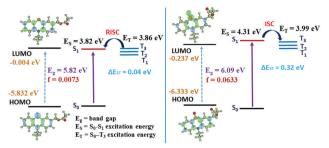
Fig. 3 The energy levels of the singlet and triplet excited states of PTZ and mono-OPTZ caged esters and the exciton decay process after photoexcitation.
