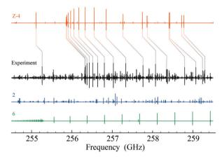
Fig. 1 Portion of the millimeter-wave spectrum around 257 GHz. The experimental spectrum (black trace) is compared with the spectral simulation of glycolaldehyde (2, blue trace), cyclopentadiene (6, green trace), and the computational guess obtained for 1.2-ethenediol (Z-4, orange trace). The intensities of the simulated spectra have been adjusted in order to match roughly the experimental spectrum.
