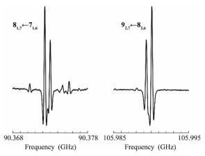
**Fig. 2** Tunneling splittings recorded for two low-frequency transitions of *Z***-4.** The observed ratio is 10:6 in accordance with spin-statistics.
