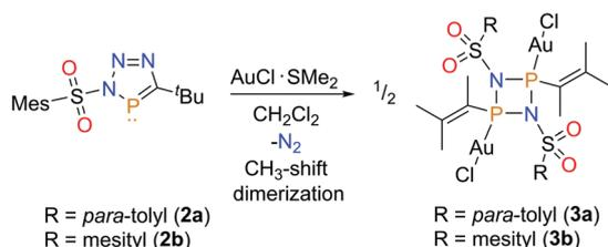
**Scheme 2** Synthesis of *cyclo*-1,3-diphospha-2,4-diazane–Au(I)-complexes **3a/b**.
