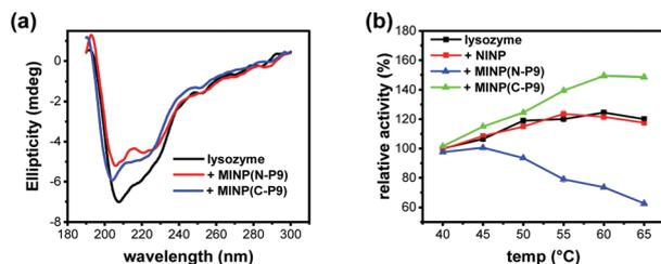
Fig. 2 (a) CD spectra of lysozyme (black) and lysozyme in the presence of 3.0 equiv. MINP(N-P9) (red) or MINP(C-P9) (blue). [lysozyme] = 0.5  $\mu$ M. (b) Relative activity of lysozyme as a function of temperature under different conditions, determined with glycol chitin as the substrate at pH 4.5 (ESI<sup>†</sup>).
