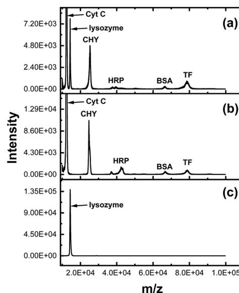
Fig. 3 MALDI-TOF MS spectra of (a) a protein mixture, (b) the remaining solution after MINP-MNP extraction, and (c) the released proteins from MINP-MNP. Cyt C = cytochrome complex; CHY =  $\alpha$ -chymotrypsin; HRP = horse radish peroxidase; BSA = bovine serum albumin; TF = transferrin. [Lysozyme] = 0.15 mg mL<sup>-1</sup>. [Other proteins] = 1.5 mg mL<sup>-1</sup>.
