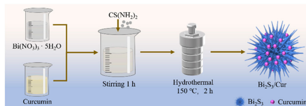
Scheme 2 Schematic diagram of \text{Bi}_2\text{S}_3/\text{Cur} hybrid material synthesis.
