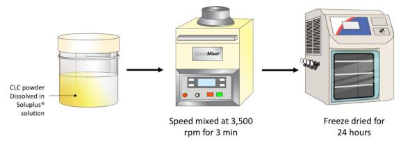
Fig. 1 Schematic illustration of the preparation of CLC-Soluplus® powders via lyophilisation.
