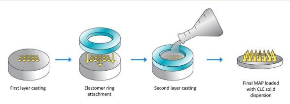
Fig. 2 Schematic illustration of the preparation of dissolving MAPs loaded with CLC.
