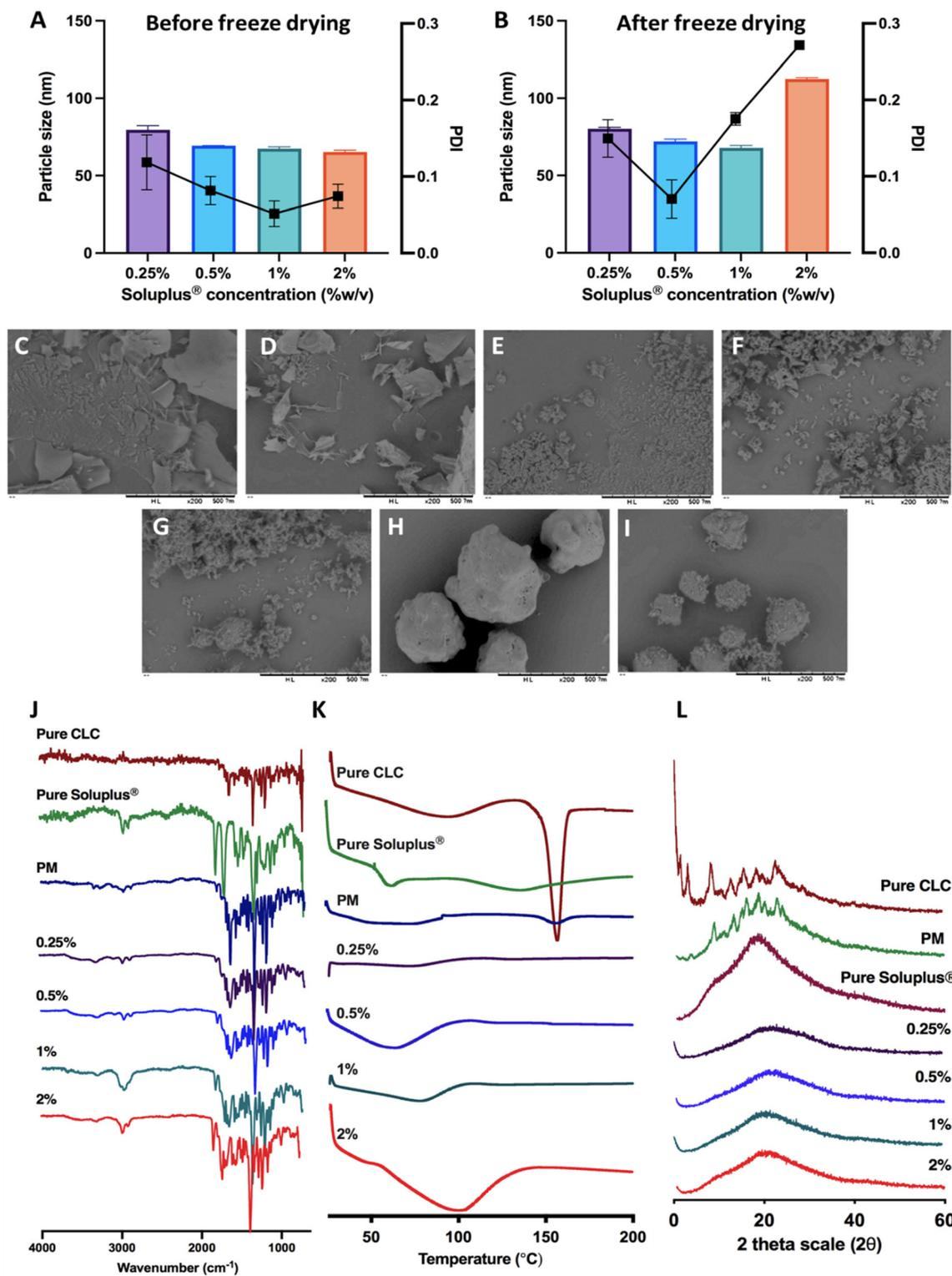
**Fig. 3** (A) Particle size and polydispersity of CLC-Soluplus® powder prior and (B) post lyophilisation (means  $\pm$  SD,  $n = 3$ ). SEM images of CLC-Soluplus® powder at different concentration of Soluplus®, (C) 0.25%, (D) 0.5%, (E) 1%, (F) 2% compared to (G) pure CLC, (H) pure Soluplus® and (I) physical mixture. (J) FT-IR spectra, (K) DSC thermogram and (L) XRD diffractogram of pure CLC, Soluplus®, physical mixture and CLC-Soluplus® powder.
