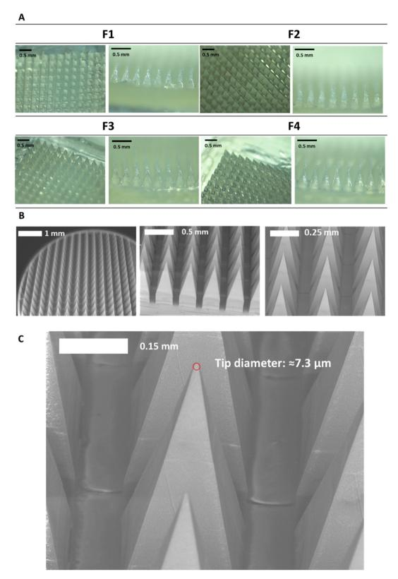
Fig. 4 (A) Optical microscopy images of CLC-Soluplus® microarray patches (MAPS) with different Soluplus® concentration fabricated via double casting method. (B) SEM images of dissolving MAPs fabricated from Soluplus® which are loaded CLC. (C) Microneedle tip diameter of CLC-loaded MAPs,  $\approx$ 7.3  $\mu$ m (n = 5).
