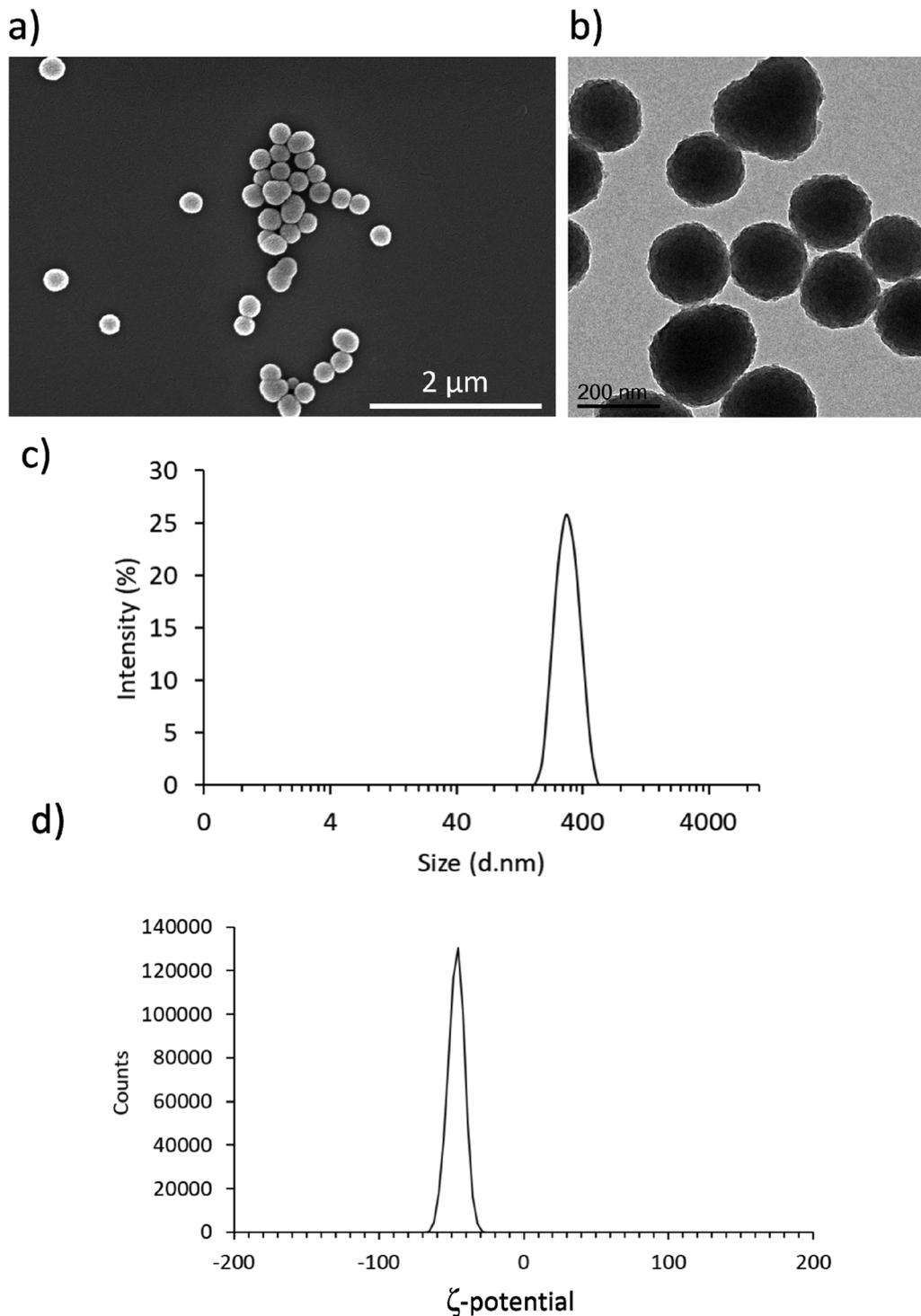
**Fig. 1** Characterization of PDNPs. Representative (a) SEM and (b) TEM images of PDNPs showing spherical morphology and uniform size. (c) Hydrodynamic diameter and (d)  $\zeta$ -potential distributions of PDNP dispersions in water.
