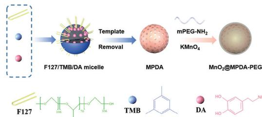
**Scheme 1** Schematic illustrations of the preparation of MnO<sub>2</sub>@MPDA-PEG NPs.
