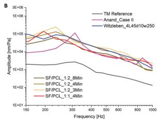
Fig. 10 The acoustic vibration curves of (A) TM implants developed in this study that have a comparable behaviour to human TM; (B) comparison of the vibration with the data from the literature (Case II<sup>27</sup> and 4L45° d10w250<sup>28</sup>).
