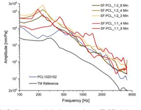
Fig. 9 Oscillatory of SF: PCL 1:1 behavior and SF: PCL\_1: 2 membranes with different spinning time.
