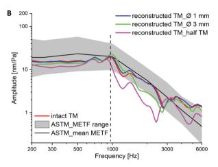
Fig. 15 (A) METF curves measured at the middle point of the footplate in temporal bone with intact TM and perforations of varying size (Ø from approx. 1 mm to half TM); (B) METF curves of the reconstructed TM after closing the perforations with the developed SF: PCL\_1: 2-membranes.
