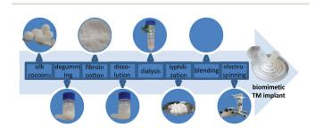
**Fig. 1** Schematic workflow from *Bombyx mori* silkworm cocoon to a TM implant with morphologically biomimetic, mechanical and oscillatory properties.
