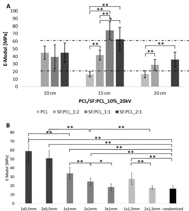
**Fig. 5** (A) Elastic moduli of PCL and SF-PCL specimens with varying spinning distance, a voltage of 20 kV and 10% concentration, dotted lines indicate the range of native TM specimens (~20–60 MPa), missing graphs indicate no spinability of the missing case group; (B) influence of oriented fibers spun with varying gap widths and number on Young's modulus of 10% PCL, 20 kV, 20 cm; \*  $p < 0.05$ ; \*\*  $p < 0.01$ .
