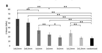
Fig. 5 (A) Elastic moduli of PCL and SF-PCL specimens with varying spinning distance, a voltage of 20 kV and 10% concentration, dotted lines indicate the range of native TM specimens (~20-60 MPa), missing graphs indicate no spinability of the missing case group; (B) influence of oriented fibers spun with varying gap widths and number on Young's modulus of 10% PCL, 20 kV, 20 cm; \* p < 0.05; \*\* p < 0.01.
