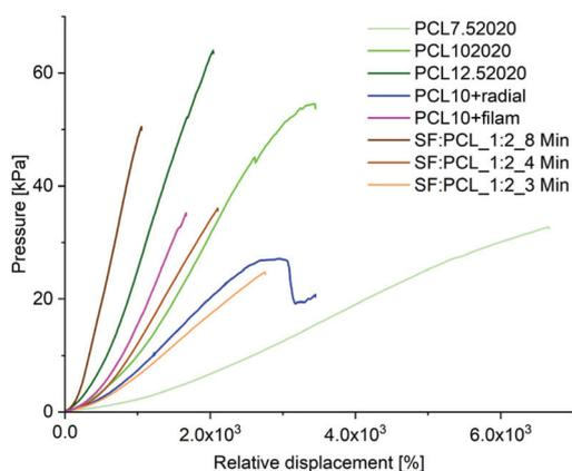
Fig. 11 Pressure/relative displacement curves of selected TM implants.
