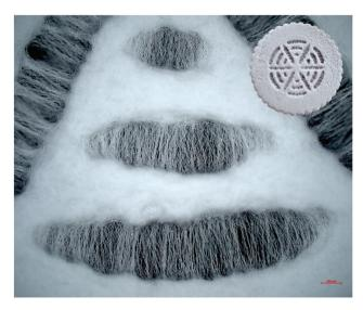
Fig. 4 Light microscopy image of radially and circumferentially oriented fibers in TM-sized membrane (scale bar 200  $\mu$ m) and whole membrane design ( $\oslash$  10 mm, top-right corner).
