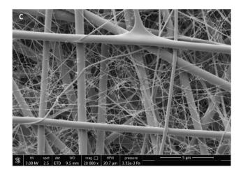
Fig. 3 (A) Fiber diameter of PCL specimens with 7.5/10/12.5%, 10/15/20/25 kV and 20 cm spinning distance; (B) fiber diameter of SF–PCL specimens with 0/33/50/66% SF, 10% polymer concentration, 20 kV and 15 cm spinning distance (large fiber fraction); (C) SEM image of SF–PCL 1:2, 10%, 20 kV, 15 cm with bimodal fiber diameter distribution, scale bar 5  $\mu$ m; \*\* p < 0.01.
