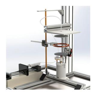
**Fig. 2** Modified electrospinning setup enabling the preparation of biomimetic TM implants with rotation unit and additional electrodes for electric field manipulation.
