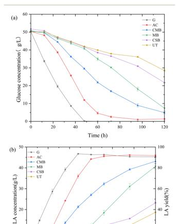
Fig. 4 LA fermentation results of prehydrolysate with different biochar detoxification. (a) Glucose consumption rate changes with time. (b) Lactic acid concentration and yield change with time.
