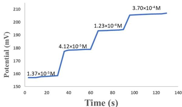
Fig. 6 Dynamic response curve of the optimized sensor no. 23.
