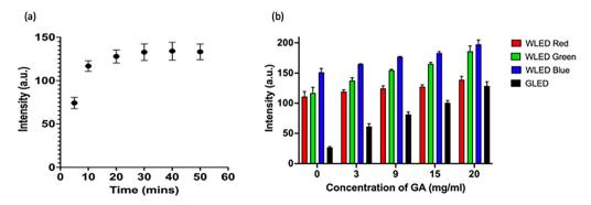
Fig. 3 (a) Development of colorimetric assay response signal intensity over time (n = 3); (b) colorimetric intensities of R-G-B channels (white LED) and green channel (green LED).
