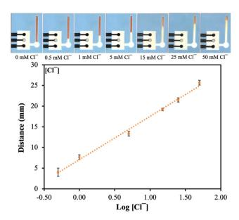
Fig. 4 The figure of a simultaneous device after detected chloride and calibration graph representing the relationship between the logarithm of  $Cl^-$  concentration (mM) and color band length (mm) (n = 6).
