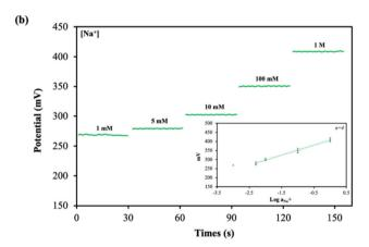
Fig. 3 Potentiometric responses of (a)  $K^+$ -ISE and (b)  $Na^+$ -ISE to varying activity of  $K^+$  and  $Na^+$  ions, respectively. The inset shows a linear relationship between the potential and the logarithm of (a)  $K^+$  and (b)  $Na^+$  activity in 0.1 M HEPES buffer pH 7.4 (n=4).
