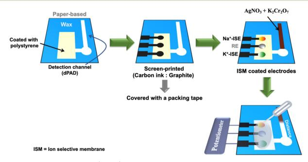
Fig. 1 Schematic illustration of simultaneous K<sup>+</sup> and Na<sup>+</sup> detection on the ion-selective electrode (ISE) and Cl<sup>-</sup> detection on the distance-based paper device (dPAD).
