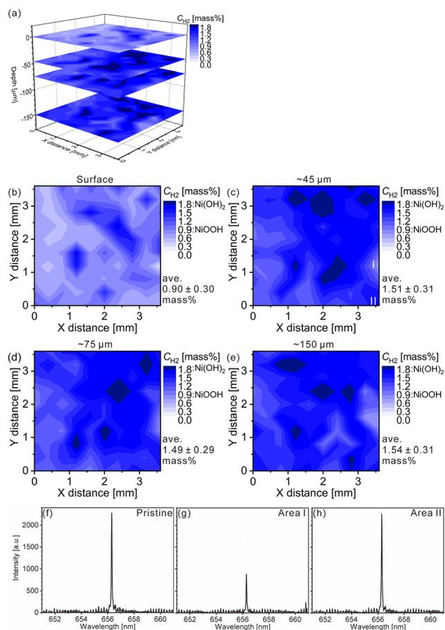
**Fig. 3** LIBS maps of the hydrogen concentrations (mass%) in the model cathode after the fifth charging for (a) 3D illustration and 2D illustrations of the (b) first layer, (c) third layer (~45  $\mu$ m in depth), (d) fifth layer (~75  $\mu$ m in depth), and (e) tenth layer (~150  $\mu$ m in depth). LIBS spectra of (f) the pristine cathode of the third layer and the model cathode after the fifth charging for areas (g) I and (h) II in Fig. 3(c).
